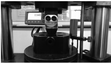
图 8 弹性轴承的压缩刚度试验和扭转刚度试验 Fig.8 Compression stiffness test and torsion stiffness test of elastomeric bearing
